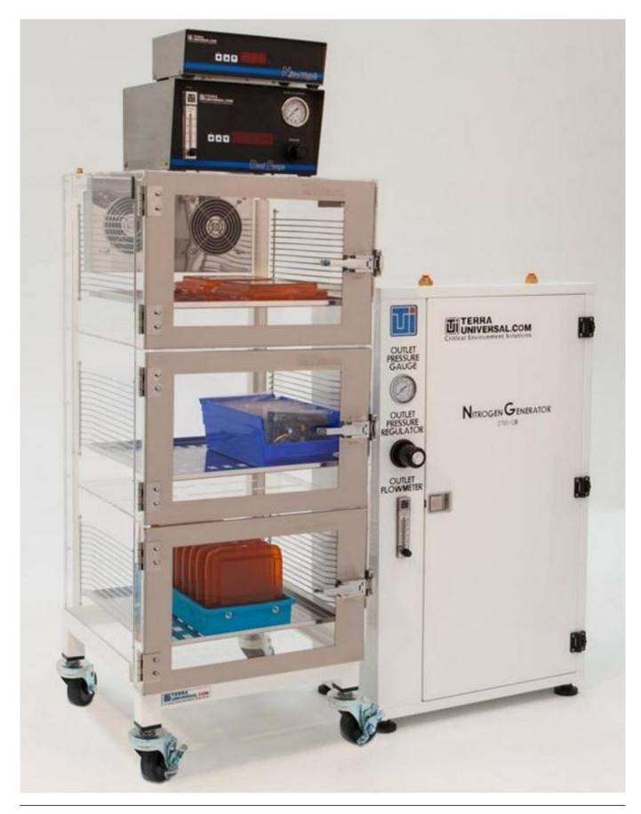
New from Terra Universal are their IsoDry Desiccators cabinets, designed to increase efficiency of low relative-humidity storage. This patent-pending design features a gas dilution module that automatically mixes internal air with nitrogen, or other process gas, to reach the programmed set-point.
