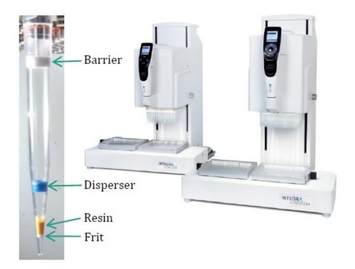
INTEGRA, in conjunction with DPX Labs LLC, has produced an application note that describes a novel high throughput semi-automated sample method for processing urine samples ready for drugs of abuse analysis by LC-MS/MS.
